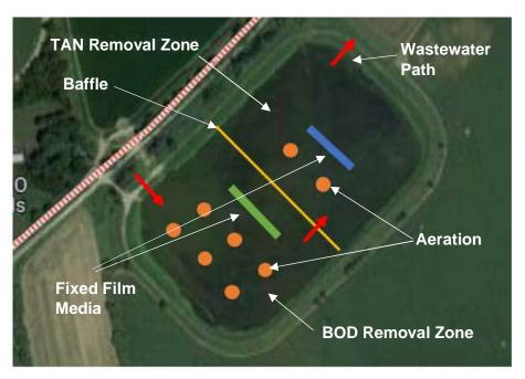
Figure 3.5 Fixed Film Treatment Example Layout
