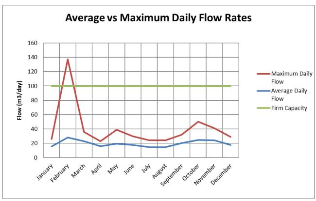
Hickson Water System Firm Capacity 100 m<sup>3</sup>/day Hickson Water System Supply Capacity 300 m<sup>3</sup>/day
