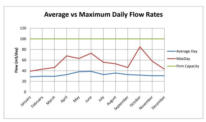
Beachville Water System Firm Capacity 100 m³/ day Beachville Water System Supply Capacity 656 m³/ day
