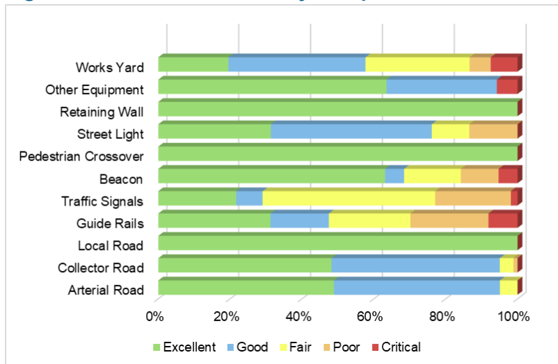
Figure 2.4.1 Asset Condition by Component
