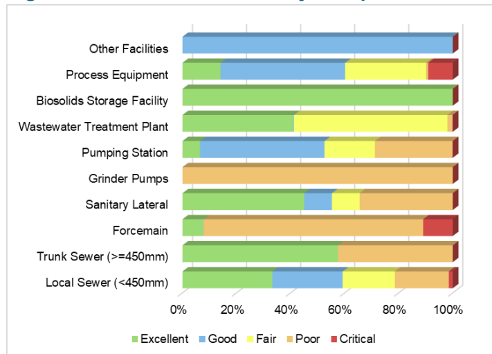
Figure 2.4.1 Asset Condition by Component
