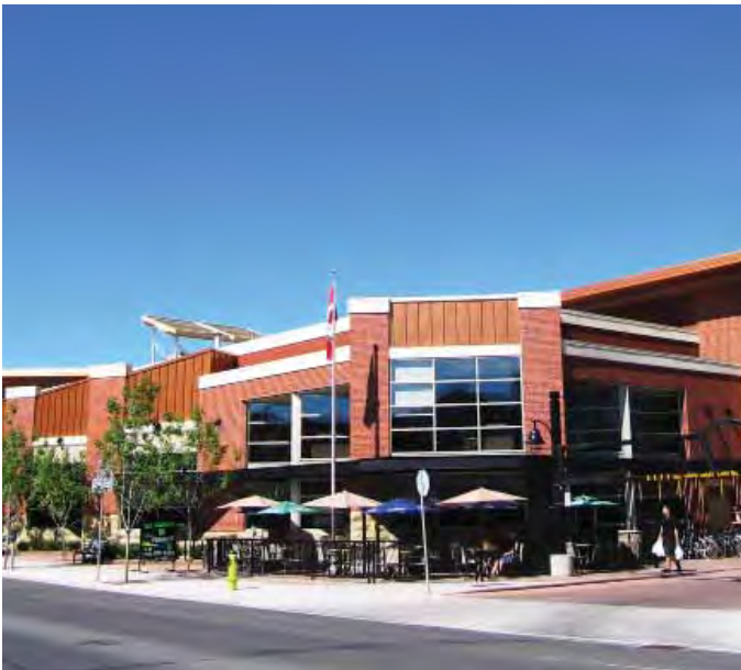
All street frontages should contain storefront glazing and entrances that are reflective of the areas fine grain fabric. Expansive blank facades are strongly discouraged.
