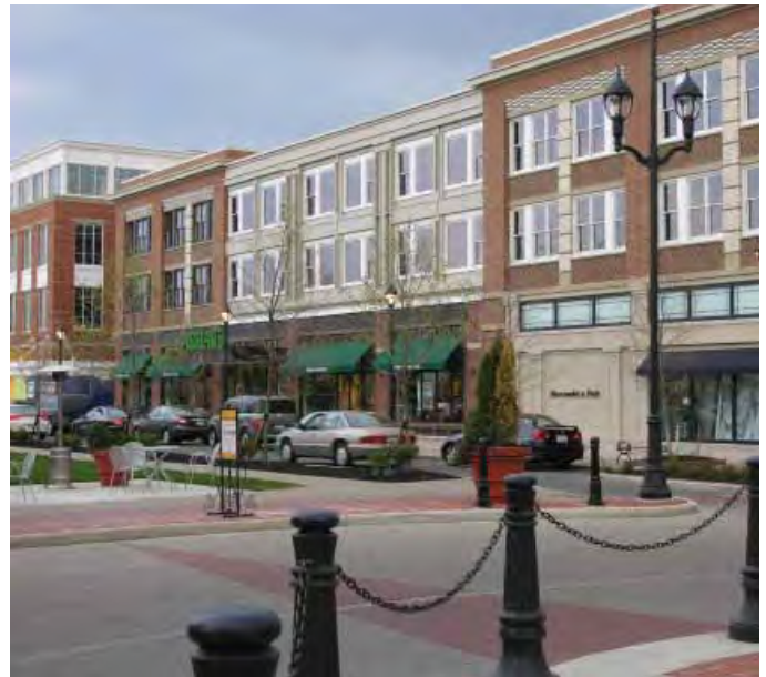
Sidewalks should be provided along the full length of the building along any facade including a store entrance and abutting public parking areas.
