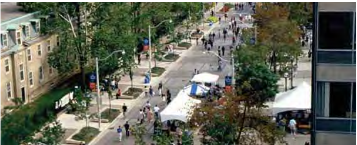
The boulevard provides a buffer between the sidewalk and vehicular traffic. The boulevard contains planted and hardscaped areas with the potential for site furnishings such as benches and bicycle locks.
